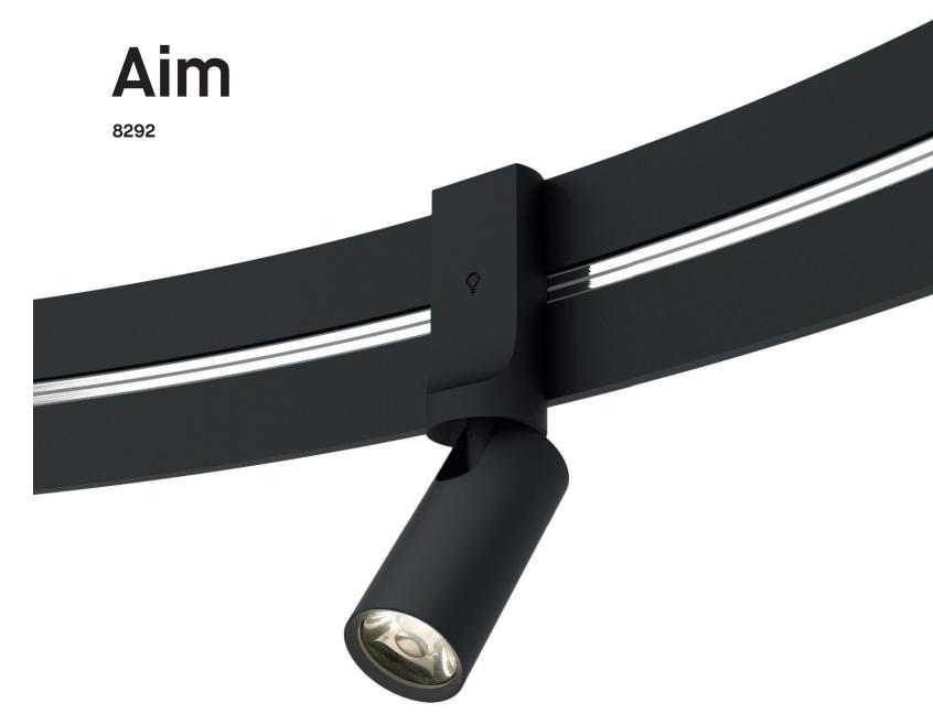
Aim is a discreet 38mm diameter aimable projector. The head rotates 350° and can be tilted up to 90° inward or outward for a wider lighting surface area. Aim can also be flipped vertically on the ring to enable direct or indirect illumination and is offered in two beam angles. A maximum of up to 12 Aim projectors can be installed on each Arena or combined with other light sources.
