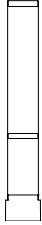
428X-P04 ONE 7" SPACER AT THE FIRST THIRD OF THE TOTAL HEIGHT. SHOWN WITH A REC1-07 CANOPY.
